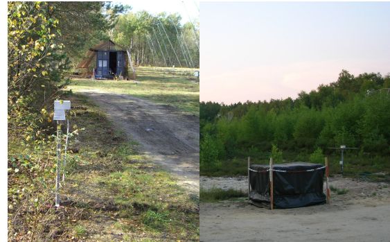
Fig. 2: A dipole near the central container located on the south side of the DAM (left). A dipole antenna and a scintillator station (right).
