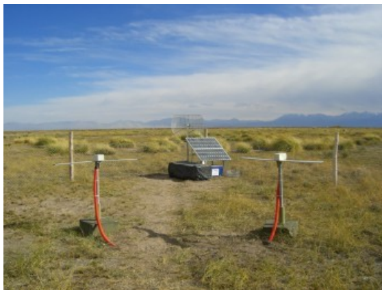
Fig. 3: Picture of a station. The electronics is placed inside the box on side of the solar panel in background. On foreground, the two dipoles in crossed polarization, identical to those used in CODALEMA.
